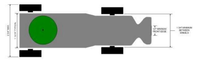
Race cars may be no wider than 2 3/4 (2.75) inches and have inside wheel to wheel clearance of at least 1 3/4 (1.75) inches. The entire car must stage behind the starting pin. The front of the car should have a 1/2" flat surface so it may be accurately placed against the starting pin. (Rule T-4) & (Rule T-9)
